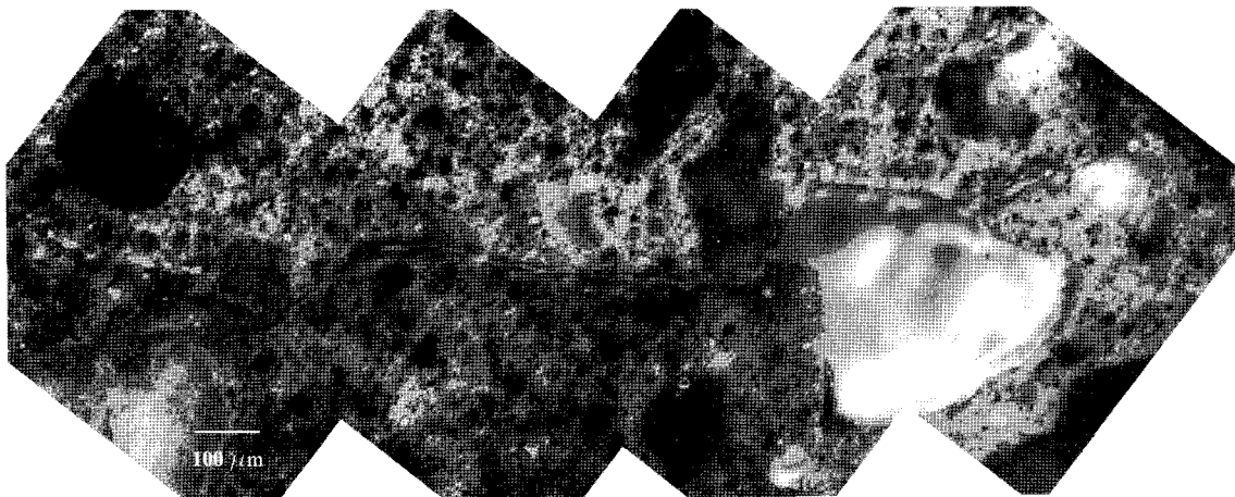
Fig. 2 Micrograph of opal aggregates exposed to 1N NaOH solution for 32 days in control specimen; ASR rim is present around opal aggregates; microcracks are filled with extruded gel
