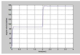
Fig. 3. The plot of angular velocity of rewind roll with proposed method
