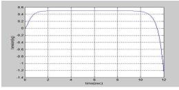
Fig. 5. The plot of tension of web with linearization at  $w_r = 87.5$  rad/sec
