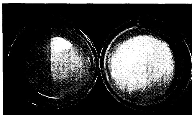
Fig. 4. Appearances of 10% (v/w) gels of rice starch (RS) and pulverized rice starch (PRS) stored at 4°C for 6 days. Left, PRS; Right, RS.
