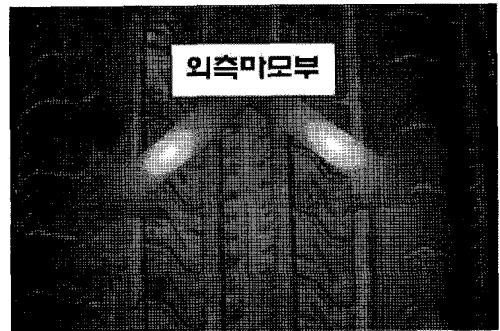
Fig. 5. Shoulder wear of a tire with a low pressure of an air in comparison to the recommended air pressure.
