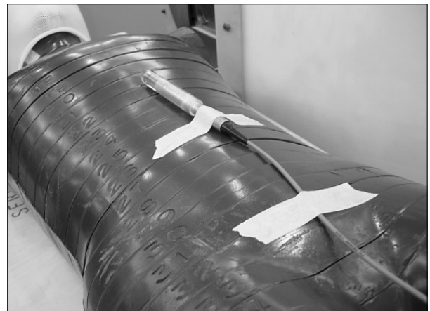
Fig. 6. Photograph of Ion chamber set-up without bolus.
