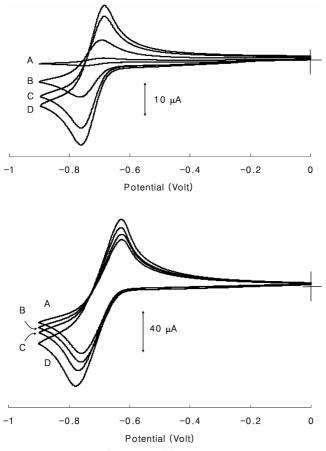
**Figure 2.** CVs of  $MV^{2+}$  diffused, from a solution containing 0.1 M  $MV^{2+}$  and 0.1 M NaCl to  $MV^{2+}$ -free NaCl solution, through Au nanotubes prepared at (A) 4. (B) 25. (C) 50, and (D) 75 °C (top) before and (bottom) after removal of a Au film on SCF. Scan rate 0.1 Vs<sup>-1</sup>.
