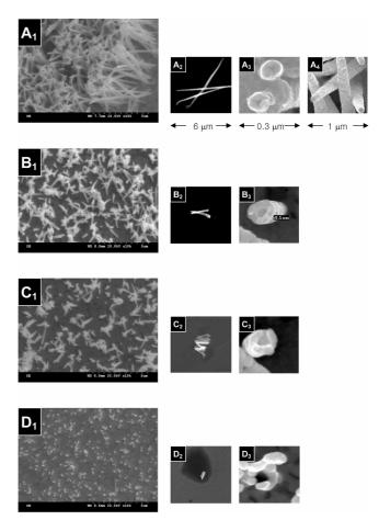
Figure 3. SEM and FESEM images of Au nanotubes prepared at (A) 4. (B) 25, (C) 50, and (D) 75  $^{\circ}$ C.
