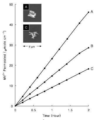
**Figure 4.** Amounts of  $MV^{2+}$  permeated through Au nanotubes prepared on solutions of  $[Au^-] = (A) 32$ , (B) 7.9, and (C) 4.0 mM at 25 °C. Insets show corresponding SEM images of nanotubes. For a SEM image corresponding to B, refer to B<sub>2</sub> of Figure 3.
