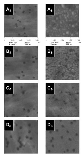
**Figure 1.** Contact-AFM images of Au-deposited membranes at (A) 4, (B) 25, (C) 50, and (D) 75 °C. Subscript a and s indicate ACF and SCF, respectively.
