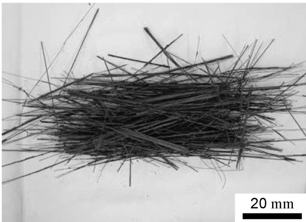
Figure 1. Photograph of bamboo fiber bundle extracted by steam explosion method.
