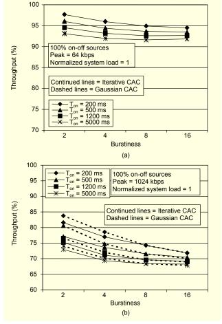
Fig. 12. System throughput over the return link: (a) PDR = 64 kbps and (b) PDR=1024 kbps.
