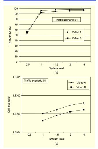
Fig. 7. (a) Return link throughput and (b) cell loss ratio for video traffic sources.
