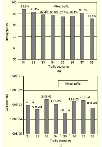
Fig. 8. (a) Return link throughput and (b) cell loss ratio in mixed condition.
