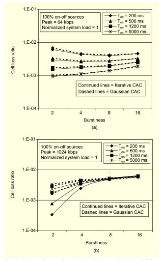
Fig. 10. CLR over the return link: (a) PDR=64 kbps and (b) PDR=1024 kbps.
