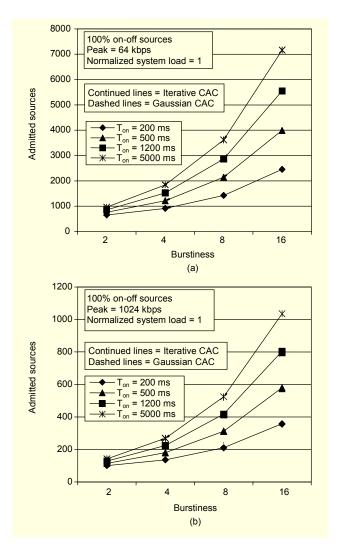
Fig. 11. Admitted sources over the return link: (a) PDR = 64 kbps and (b) PDR=1024 kbps.
