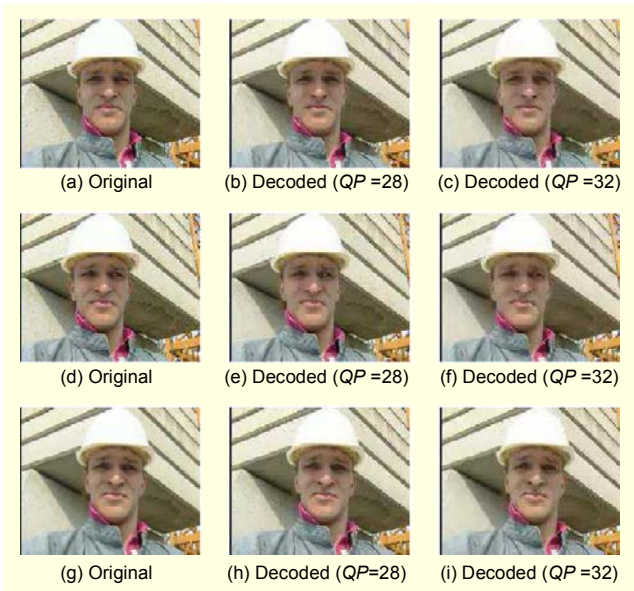
Fig. 8. Decoded images for visual comparison of the Foreman sequence (QCIF). (a)-(c): frame 10, (d)-(f): frame 25, and (g)-(i): frame 50.
