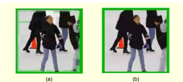
Fig. 7. Decoded results when boundary handlings for both half-pel interpolation and upsampling are (a) not handled and (b) handled (3 spatial layer).
