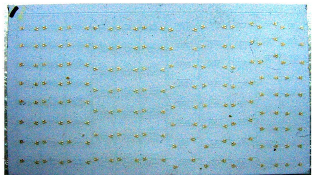
Fig. 2. LTCC test structure (only exposed top layer is visible).
