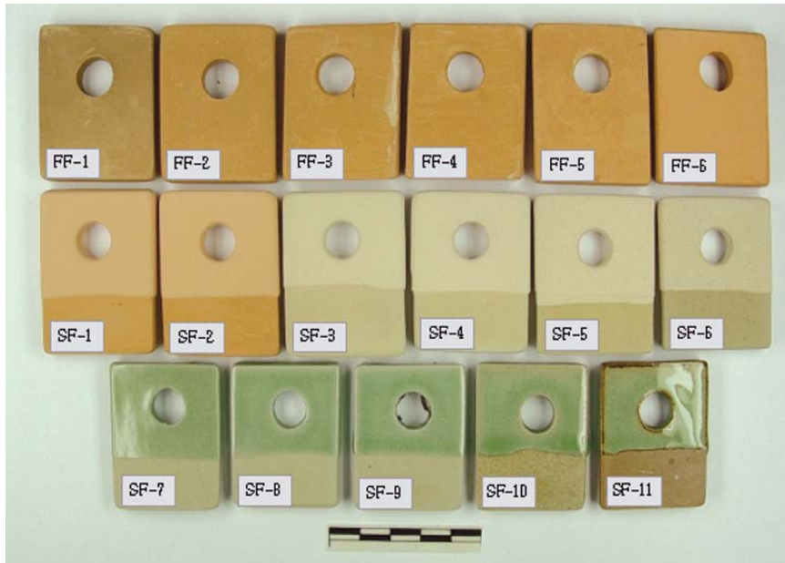
Photo 1. Samples formed with modern material and fired in gas furnace
