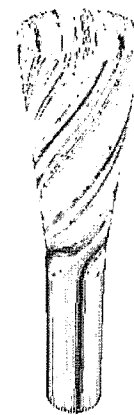
Figure 3. Typical path lines of air in Z-nozzle.
