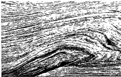
Fig. 6 The folding defect on workpiece head after ECAP
