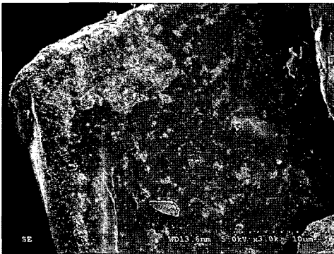
Fig. 2. SEM micrographs of \text{Fe}_{73}\text{Si}_{16}\text{B}_7\text{Nb}_3\text{Cu}_1(\text{at}\%) powder surface (a) Fe-based powder mixed with the binder of 3 wt% (b) Fe-based powder mixed with 3wt% binder, annealed to burn out of solvent at 205^\circ\text{C} (c) Fe-based powder mixed with 3 wt% binder, annealed to crystallize at 550^\circ\text{C} (d) at 650^\circ\text{C} .
