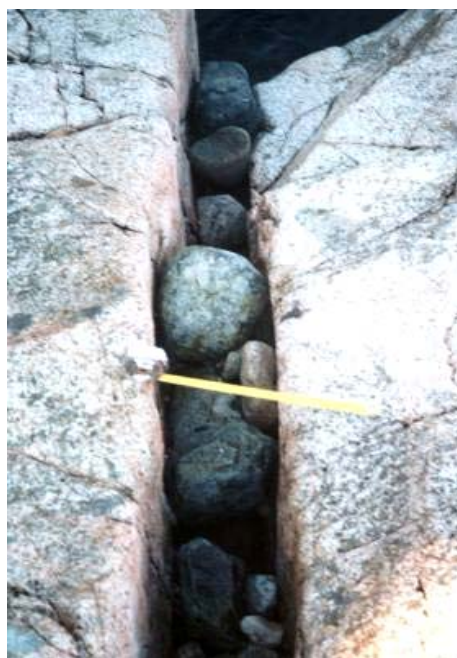
Fig. 3. Sediment particles in a crack in the River Etive. The sediment particles inside the crack are important tools for hydro-wedging (Tape shows flow direction). The yellow scale is 40 cm long. Sediment particles are stuck into the crack, so cannot be moved.
