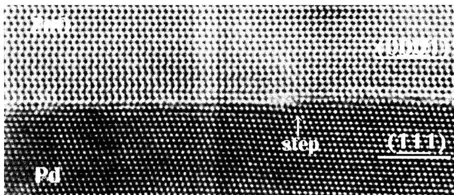
Fig. 2. Well defined ZnO/Pd interface being parallel to (0001) of Zn and to (111) of Pd. No periodic local strain contrast corresponding to a misfit dislocation is seen in the image. An atomic step is indicated by an arrow.
