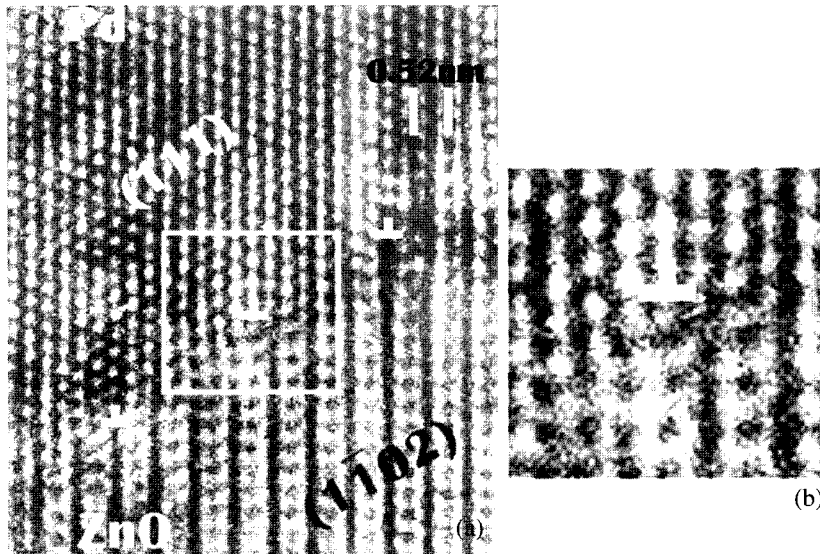
Fig. 6. Local stress accommodation of ZnO ( 1\bar{1}01 )/Pd (200) interface by putting of local strain. Local atomic displacement near the dislocation core is apparent in (b).
