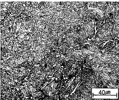
Fig. 1 As-received microstructure of A350 LF2
