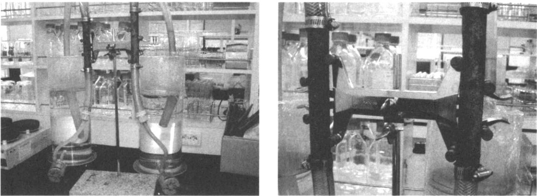
Fig. 2. Photographs of continuous loop plant for the old pipes(aged 28 years) corrosion test.
