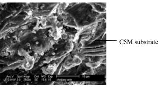
Figure 1. ESEM photo of CSM substrate not fermented (control)
