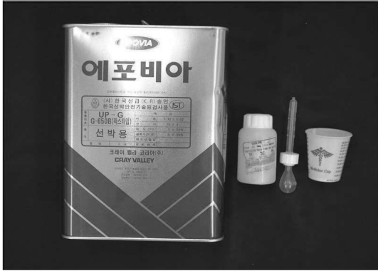
Fig. 2. Mounting media(Epovia, CrayValley Inc. Korea) and specimens which were mounted.
