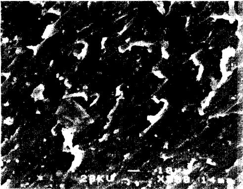
Fig. 8. SEM micrograph of the fracture surfaces of a rubber bush at load amplitude 1200kgf.
