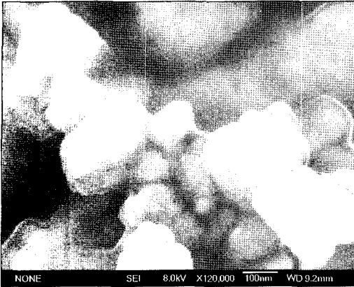
Fig. 5. Nano TiNx morphology on the surface of powders milled for 10 hours.
