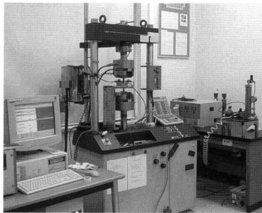
**Fig. 2.** Photograph of fatigue test machine (INSTRON 8516).
