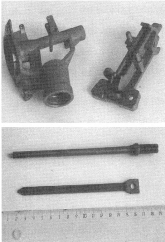
Fig. 1. Examples of mechanical parts treated by post oxidation.
