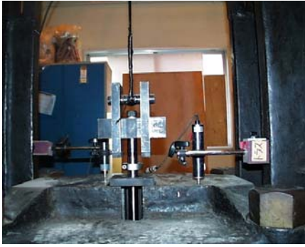
(b) Tensile test of U type anchor Photo.2. Experiment situation.
