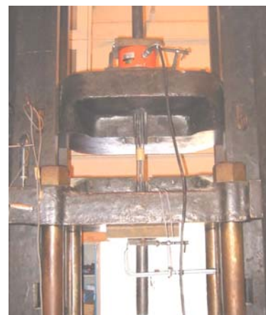
(a) Tensile test of CFRP rod
