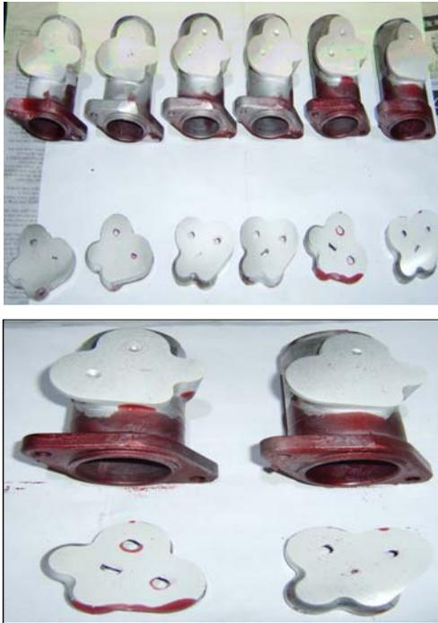
Fig. 17 An inspection of interior a blow-hole using color check.
