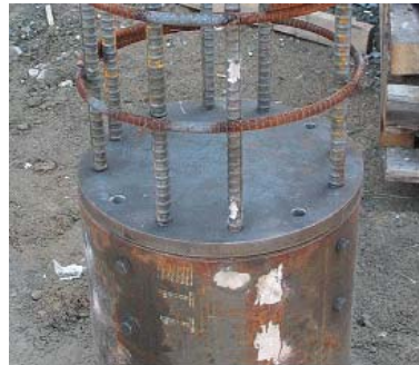
Fig. 2. Details of reinforcement for Type-A
