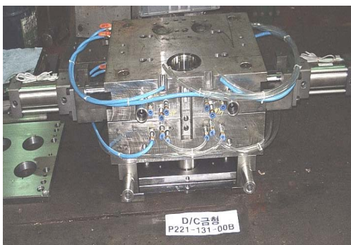
Fig. 12 Mold of Cavity Close State
