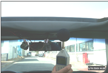
Fig. 9 Noise testing situation
