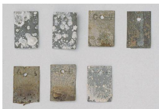
(d) The status of lead before and after the test
