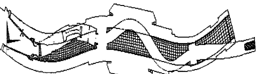
Fig. 9(f) 3rd mode shape of the spindle and drawbar [977Hz]
