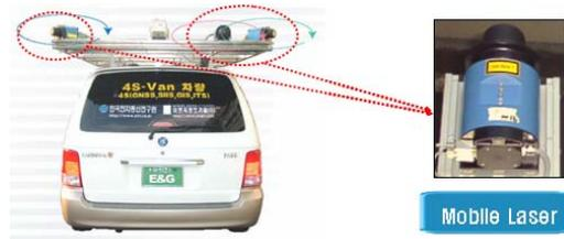
FIGURE 1. GPS-VAN laser system
