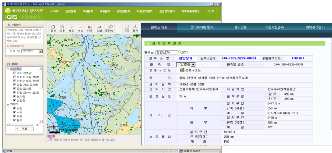
FIGURE 3. Screen of the IGIS(Integrated Groundwater Information Service System) and an example of data searching for Cheonan district
