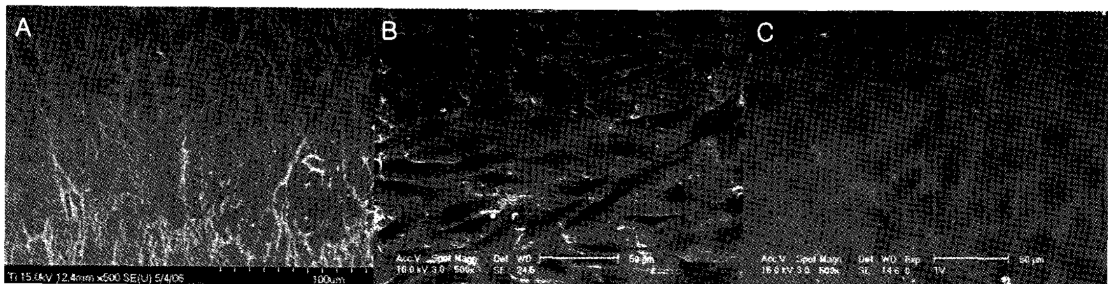
Figure 3. Photomicrographs of SEM findings at day 3. Pure Ti (A) and Ti-8Ta-3Nb (B) surfaces show that cells grown on both Ti and Ti-8Ta-3Nb surfaces, presented a flat, elongated spindle-like morphology, while cells on Ti-6Al-4V (C) surface were flat, but some cells were oval or round in shape (x 500).
