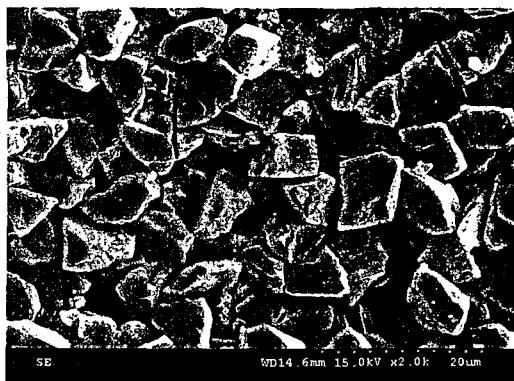
Fig. 3 SEM image of a micro-porous coated surface (Particle size:  $6\pm2 \mu\text{m}$ ).
