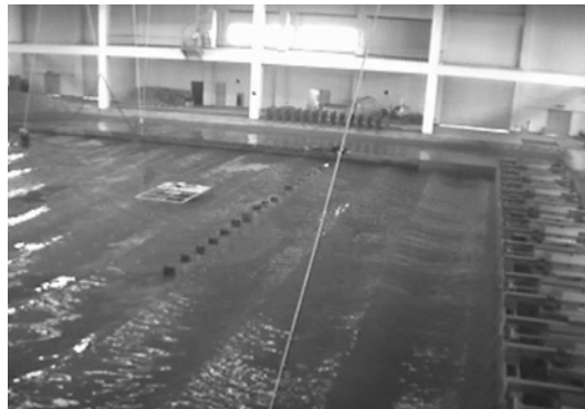
Fig. 13. Hydraulic model experiment with leodo underwater rock (S direction).
