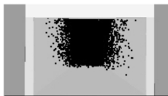
(b) No smoke spread-out through the door
