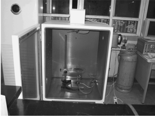
Fig. 1. Toxicity analysis apparatus of fire gases.
