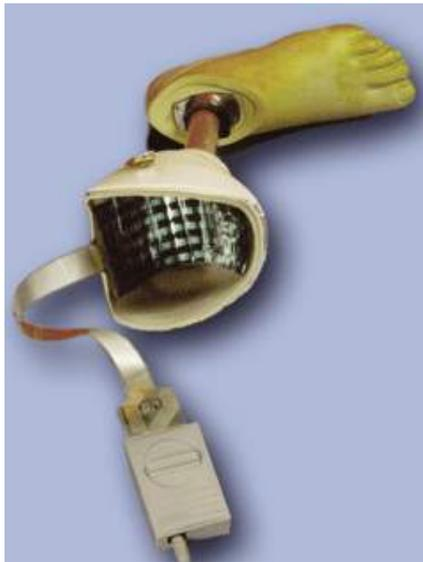
**Figure 1.** Sensors inserted in socket.
