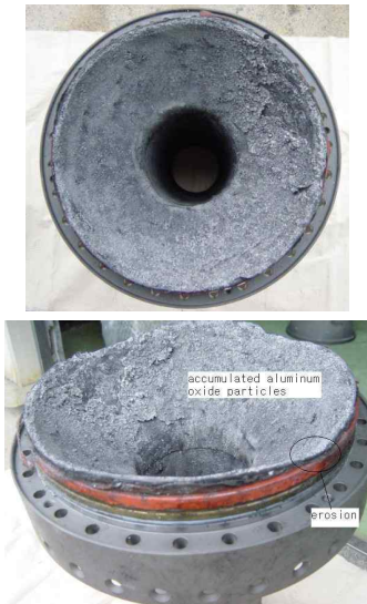
Fig. 8. Post-test views of nozzle entrance liner for propellant P showing erosion with the deposited layer of aluminum oxide
