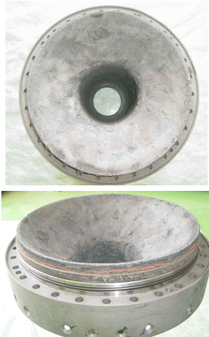
Fig. 7. Post-test views of nozzle entrance liner for propellant H
