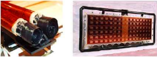
Fig. 6. Spring roll up device in SAR frame
