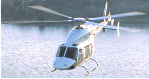
Fig. 1. Helicopter model with the skid landing gear system (SB427 by Bell Helicopter Co.)
