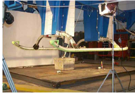
Fig. 9. Experimental drop test set-up for the level landing condition
