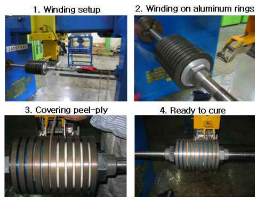
Fig. 1. Manufacturing process for composite /aluminum ring specimens
