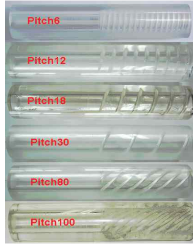
Fig. 2. Helical fuel grains used for combustion test
