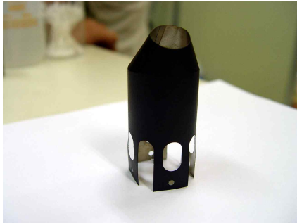
Fig. 9. Developed Radiation Heat Shield
