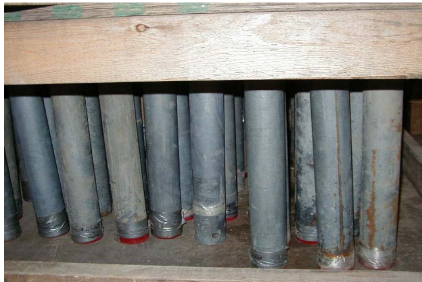
Figure 2. Vertical fixing sample transport frame (VFSF).
