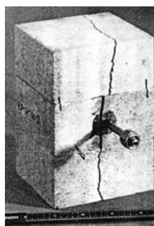
(b) Lateral offset of hydraulic fracture across an unbonded interface of limestone (Hanson et al., 1981)
