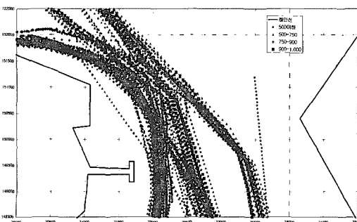
Fig. 21 The distribution of ESA on connecting areas between special sea area and No.2, 3 and 4 Fairway
