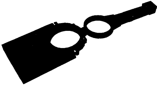
Fig. 6 Topology optimization result for maximizing compliance
